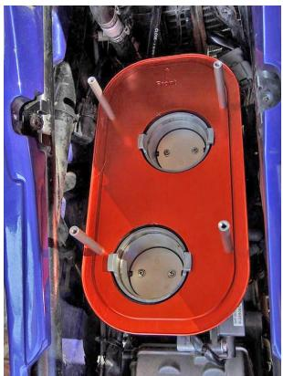
5. Install the velocity stacks in place, rotating them 45 deg. to lock.
