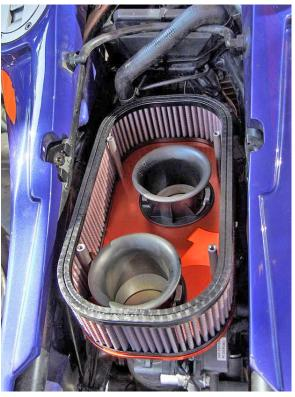
7. Install the top of the DNA S3 Air Box Kit and bolt it in place (MK3 is displayed bellow left & MK1 is bellow right)
