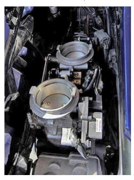
Install the DNA DN-9410-R2 NITRILE L-RINGS supplied, on the throttle bodies. Read instructions on L-RING for top side.
