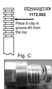
Install the stock needle retainer on top of the Dynojet needle, e-clip and washer.
