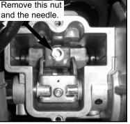
For 2007-2015 models, Remove this 8mm nut to remove the needle.
