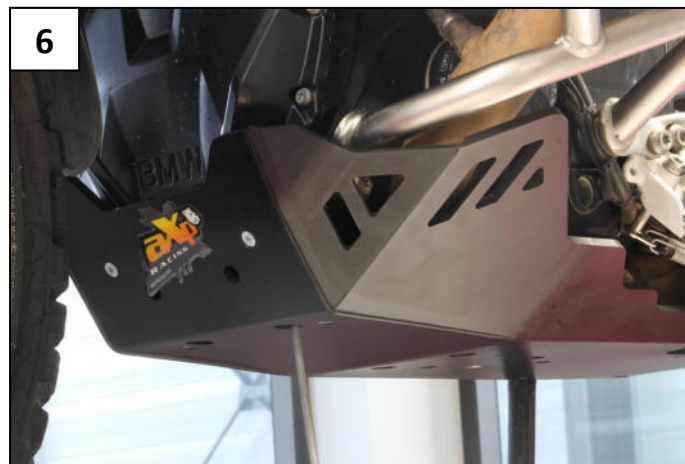
Place the front Tbhsc 8x35mm screws with M8 Washers
